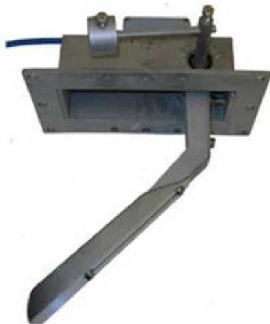
Figure 2: Flow paddle arm in the bottom position (zero flow)
